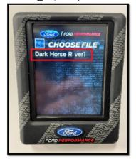
• When prompted, turn the ignition switch off, the flash is complete.
