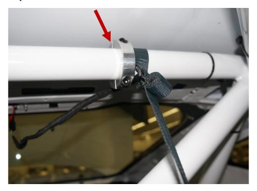
• Install 1 collar on main safety cage center area as shown
