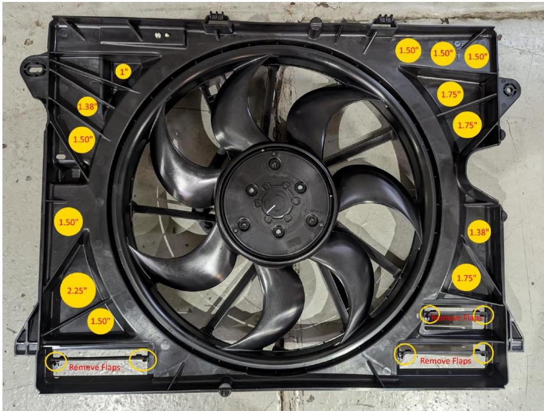
Figure 1: Material removal locations and maximum hole size
