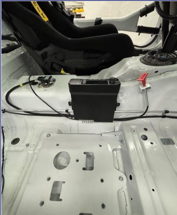
Radio Location Right Side of Drive Shaft Tunnel
