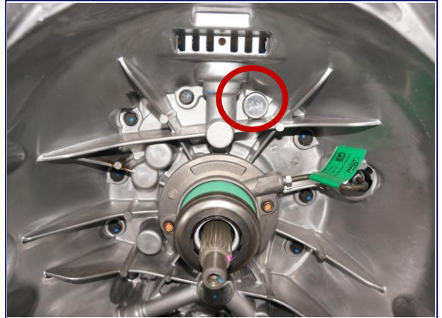
Transmission Seal 2 Inside Bell Housing
