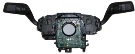
Multifunction Switch DHR-CLMNSWTCB-MOD
