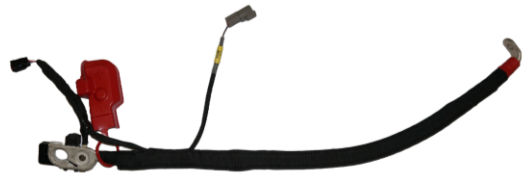
Battery to Breaker Cable FP-14B060-AA
