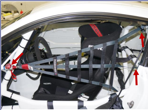
Driver Helmet Support Net Mounting Points
