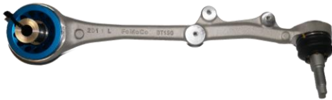
Arm LH - Lower Front Assembly DHR-FCNTRLBRNG-MOD
