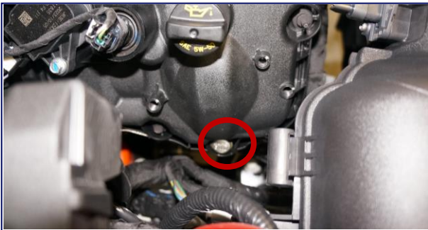
Engine Seal 3 Valve Cover RH Seal
