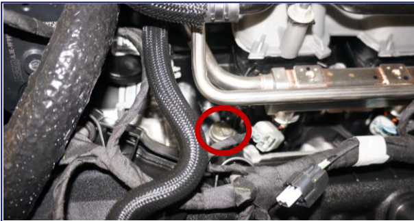
Engine Seal 4 Intake Manifold Seal
