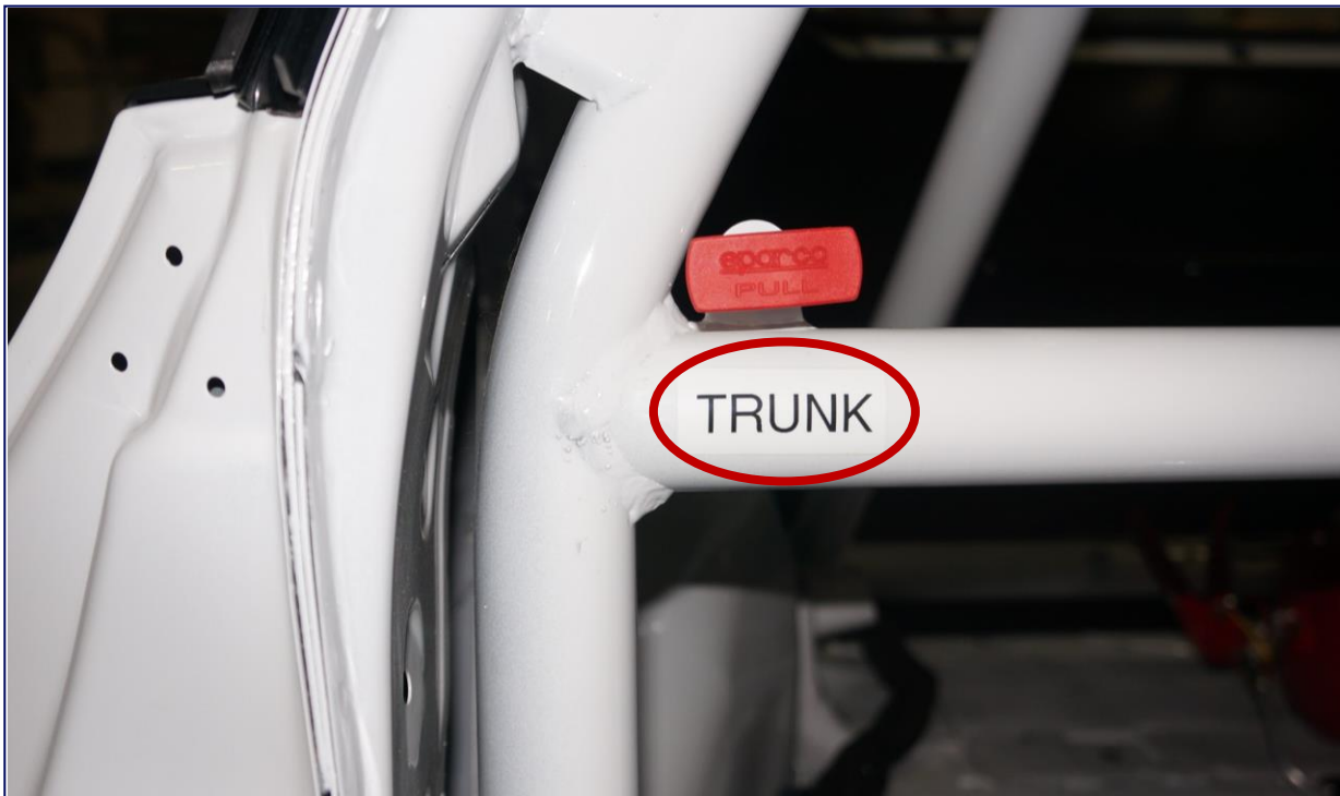
Trunk Release Handle – Must be clearly labeled –
