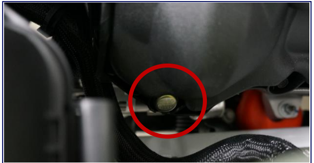
Engine Seal 2 Valve Cover LH Seal
