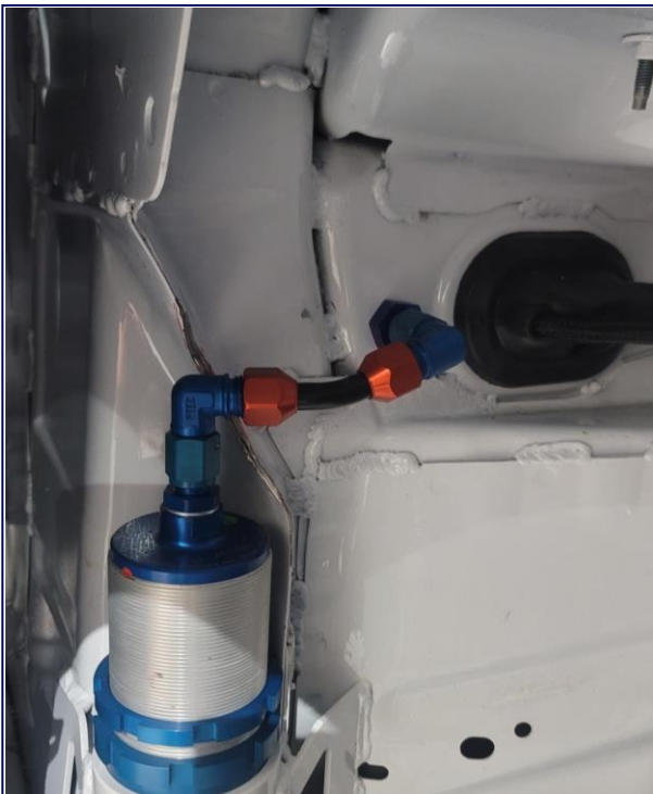
Front Air Jack / Bulkhead Connection Passenger Side
