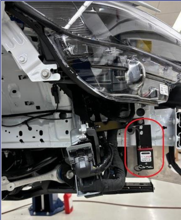
Transponder Location Front Passenger Side
