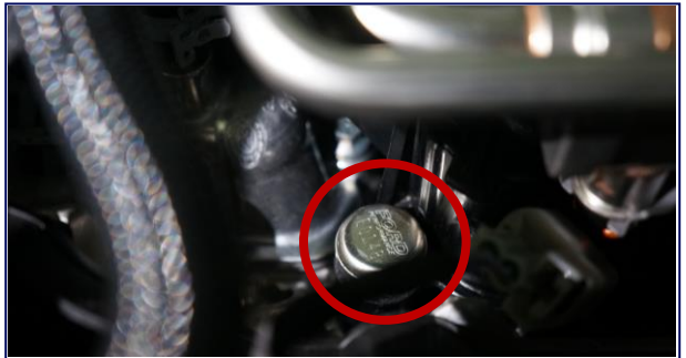
Engine Seal 4 Intake Manifold Seal
