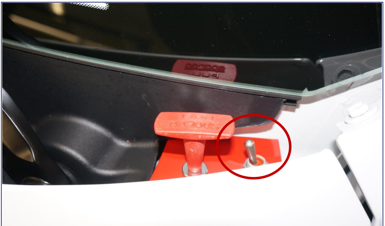
Exterior Master Power Electrical Switch Exterior Driver Side
