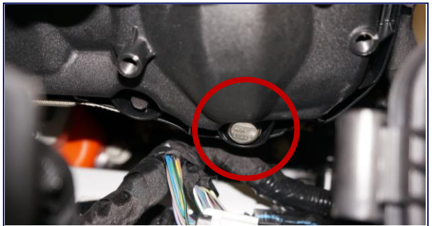
Engine Seal 3 Valve Cover RH Seal
