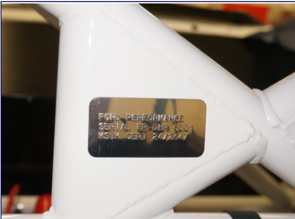
Chassis Serial Number – Safety Cage Tag Standard (As Delivered)
