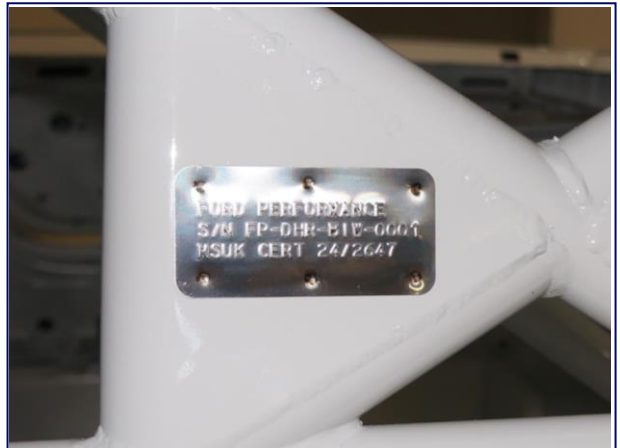
Chassis Serial Number – Safety Cage Tag BIW
