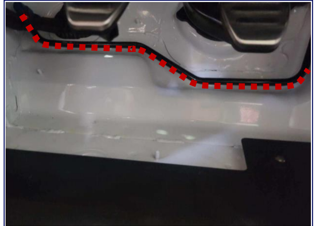
Front Air Jack Line Routing Driver Side
