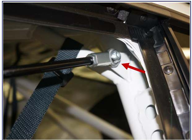
Driver Window Net Rod Mounting Point
