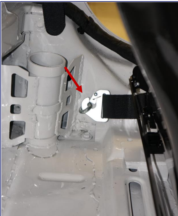
Harness Mounting Point Driver's Side Rear
