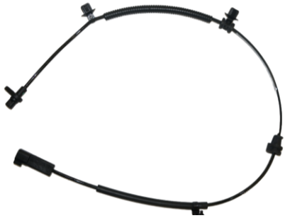
ABS Sensor - Front LH JR3C-2C204-B1B
