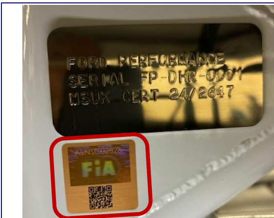
Safety Cage FIA Certification Standard (As Delivered)
