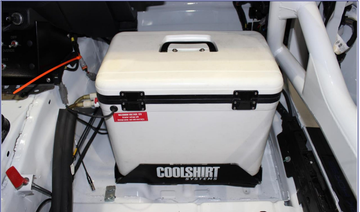
Driver Cooling System Location Passenger Side Footwell
