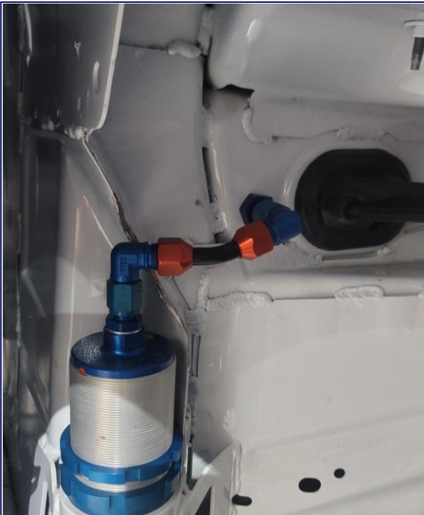
Front Air Jack / Bulkhead Connection Passenger Side
