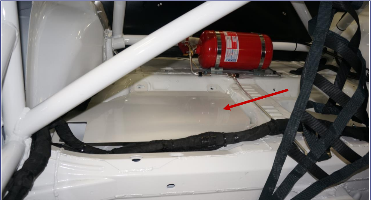
Optional Driver Cooling System Mount* 13052-09-1158 Passenger Side Rear Seat *Mount will be zinc-plated
