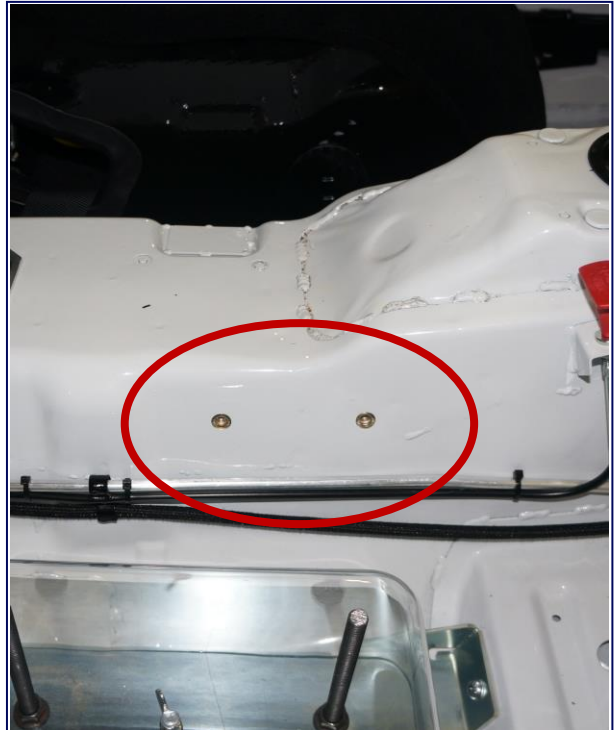
Radio Mounting Location (2) M6 Rivnuts Provided
