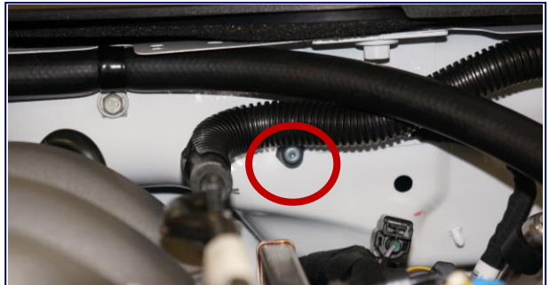
Engine Bay Nozzle 1 Driver Side
