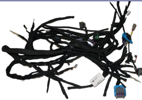
IP (Dash) Harness, Modified PR3T-14401-EEMOD
