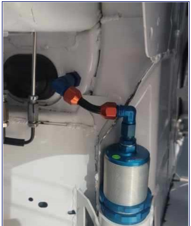
Front Air Jack / Bulkhead Connection Driver Side
