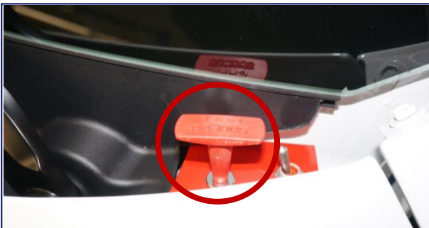
Exterior Cable Pull Exterior Driver Side
