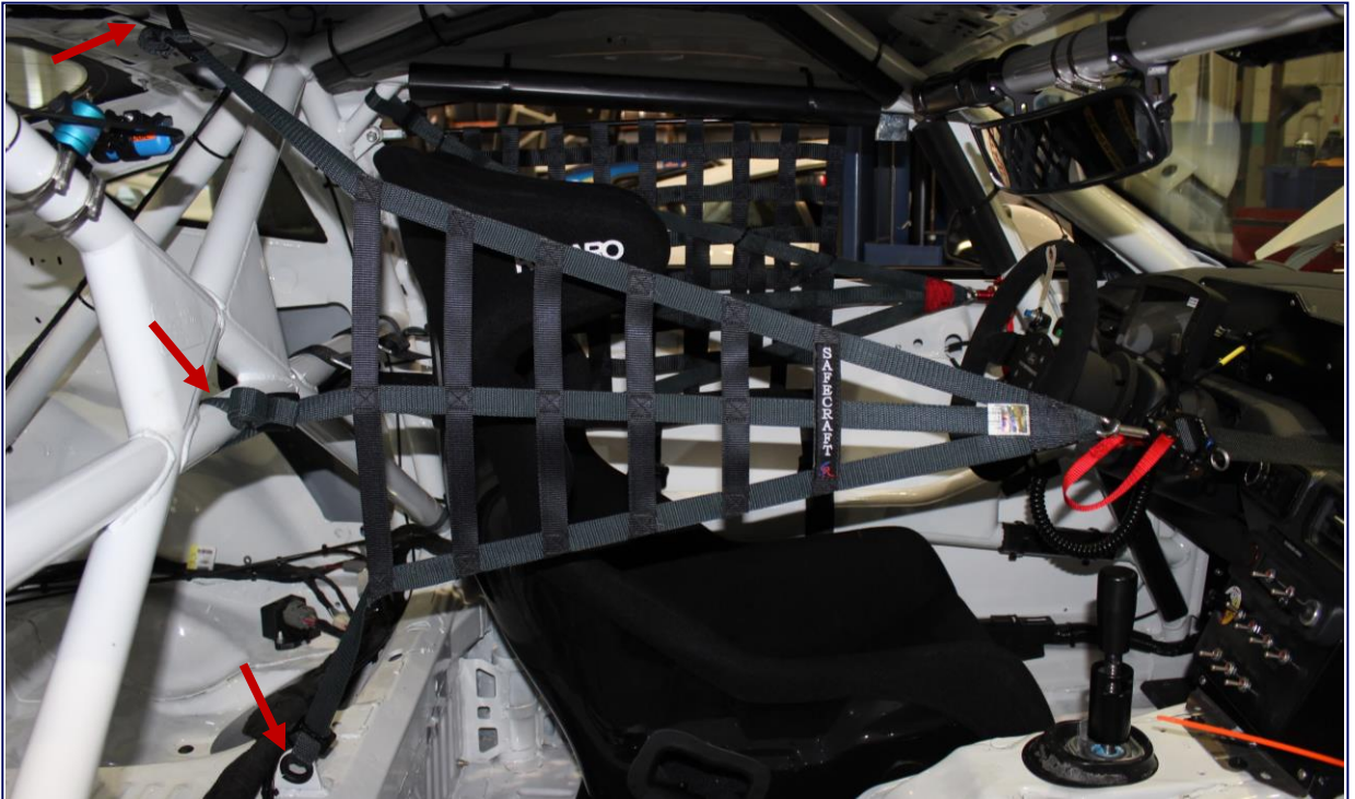
RH Helmet Support Net (Ratchet Release) Mounting Points
