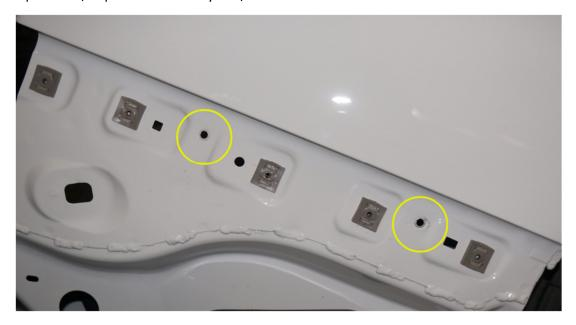
Install the four Quik-Latch studs only using a washer on the inside of the body.
