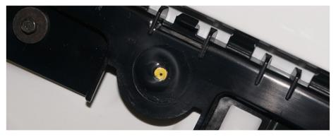
Mark and drill the dimples with a 1/8" pilot through the bracket. Continue through the sheet metal, two per side.
