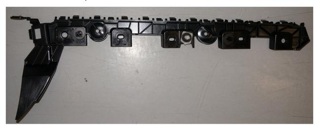
Snap bracket onto Fascia and drill 1/8" pilot hole through the fascia
