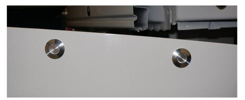
Reinstall fascia and adjust studs to desired length
