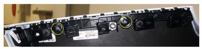
Remove brackets from fascia and open the 1/8" holes to 3/4"  $\,$
