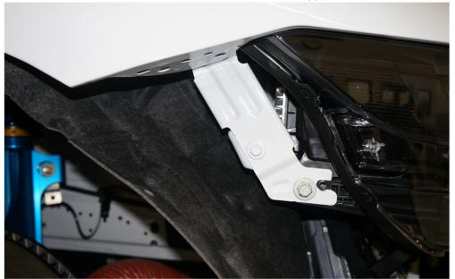
Center punch for the Quik-Latch on the center rib 1 3/8" down from the top
