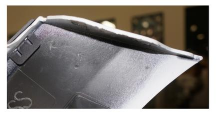
Align the fascia back on the vehicle in the production position, then tap on the fascia over the Quik-Latch ball end stud with the palm of your hand to dimple the back of the fascia where the Quik-Latch is to be installed
