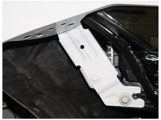
Install Quik-Latch long stud where the head of the stud is just flush with the fender.
