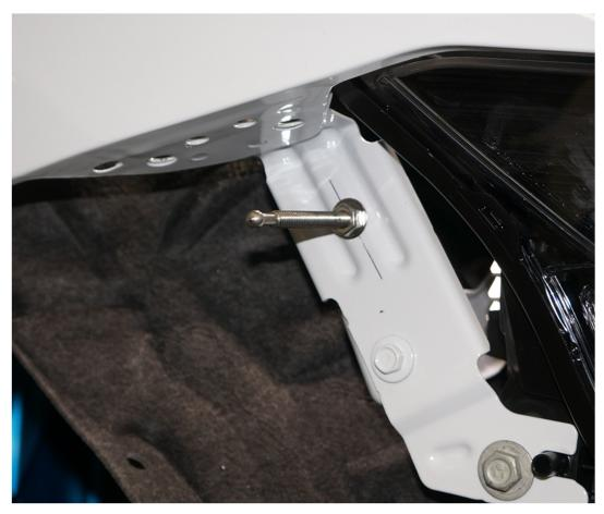
Remove fascia to fender bracket by pulling push pin
