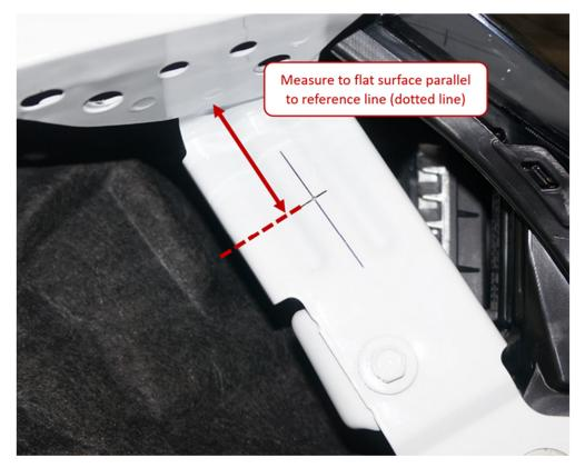
Drill a 1/8" hole in the center rib 1 3/8" down from the top
