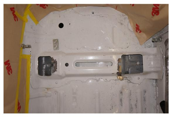
Remount the plate with the M10  $\times$  1.5 flat socket head cap screws, slide to center of vehicle and tack in place using the three included gussets.
