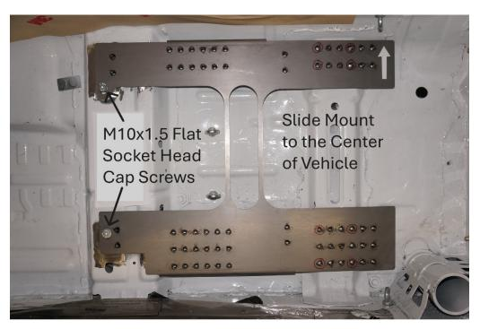
Once the mount is temporarily installed, using a transfer punch, mark the eight holes shown below on rear factory seat mount crossmember.
