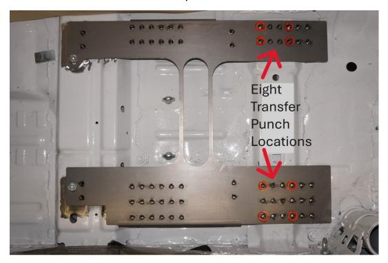
Remove the mounting plate and drill the marked locations with a 7/8" Drill.
