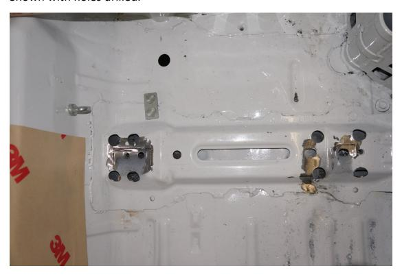
Cut the centers out on each side for clearance to the weld nuts on the back side of the seat mounting plate.
