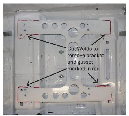
Once the bracket is removed, open the two marked holes on the front factory seat mount crossmember with a 7/8" drill for clearance to the weld nuts on the back of the seat mounting plate.
