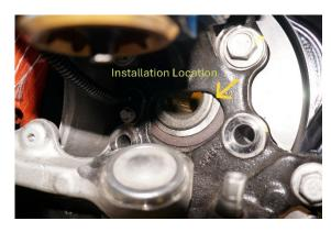
Install with a small bead of high temperature silicone.
