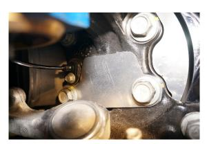
Use standard torque for front bearing assembly, 150 Nm.
