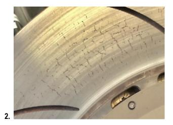
A rotor that has been used and / or run at a higher temperature range will exhibit "stress cracks" on the rotor outboard and inboard surfaces only (picture 2, above right). Continued use will cause these "cracks" to grow in length, which is considered normal. If the cracks propagate around the OD or the ID of the rotor then it is considered no longer usable and must be changed.
