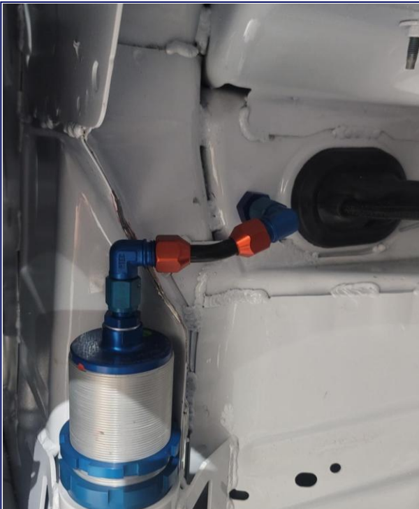
Front Air Jack / Bulkhead Connection Passenger Side
