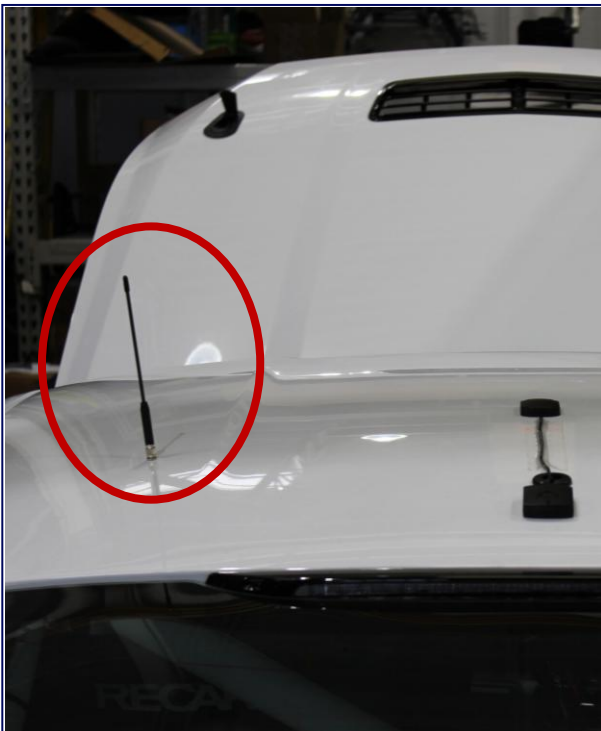
Radio Antenna Location Driver's Side Roof Panel
