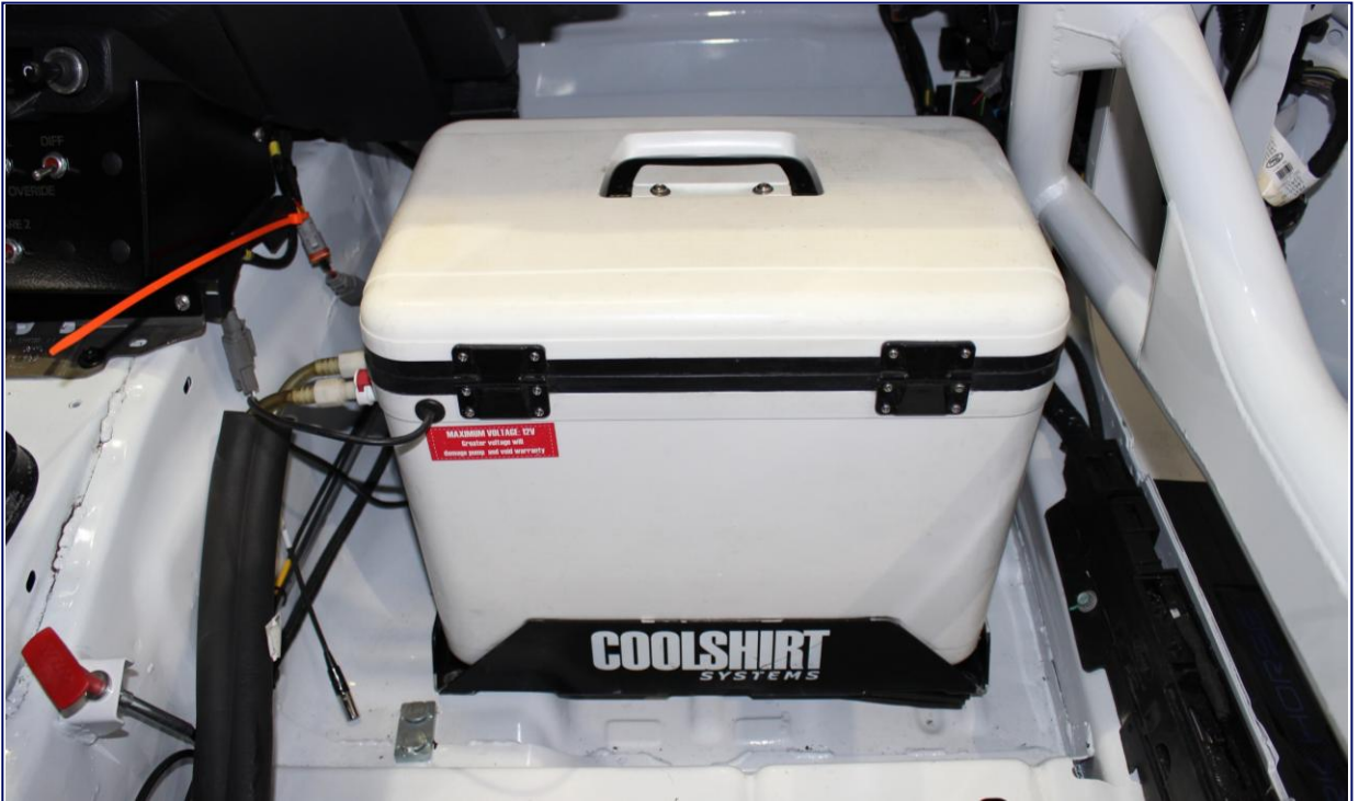
Driver Cooling System Location Passenger Side Footwell
