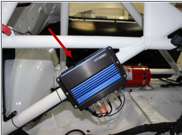
VBOX Mount Location Option 1 Passenger Side Roll Cage
