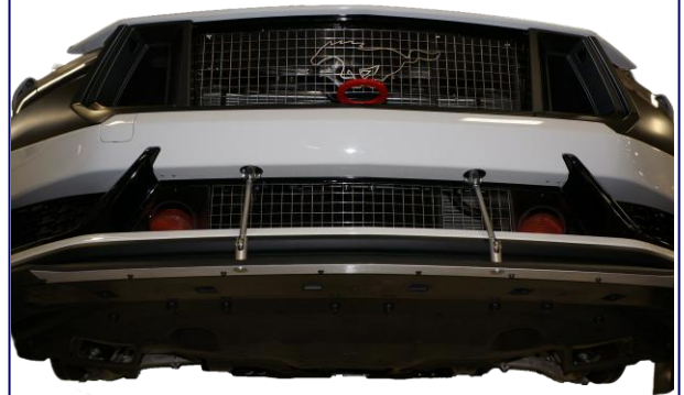
Splitter Support Assembly
