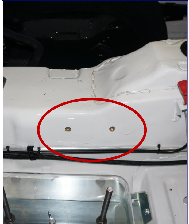
Radio Mounting Location (2) M6 Rivnuts Provided
