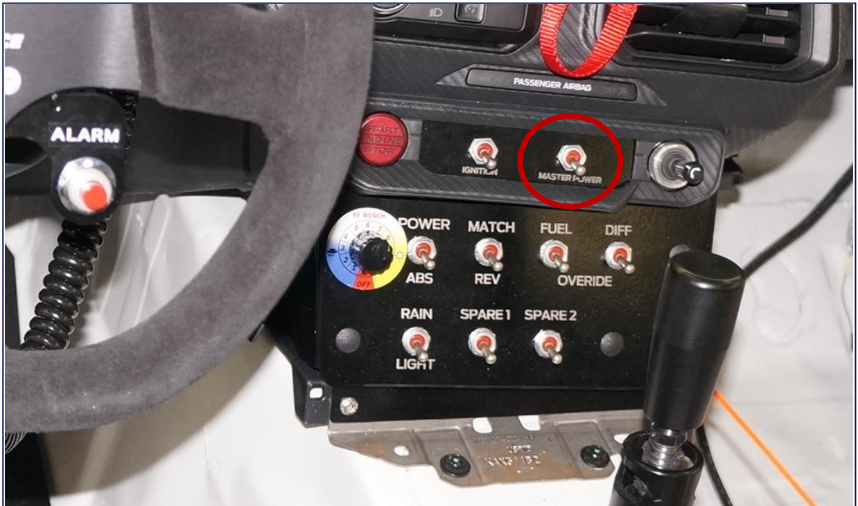
Interior Master Power Electrical Switch OFF – Down towards Floor / ON – Up towards Roof
