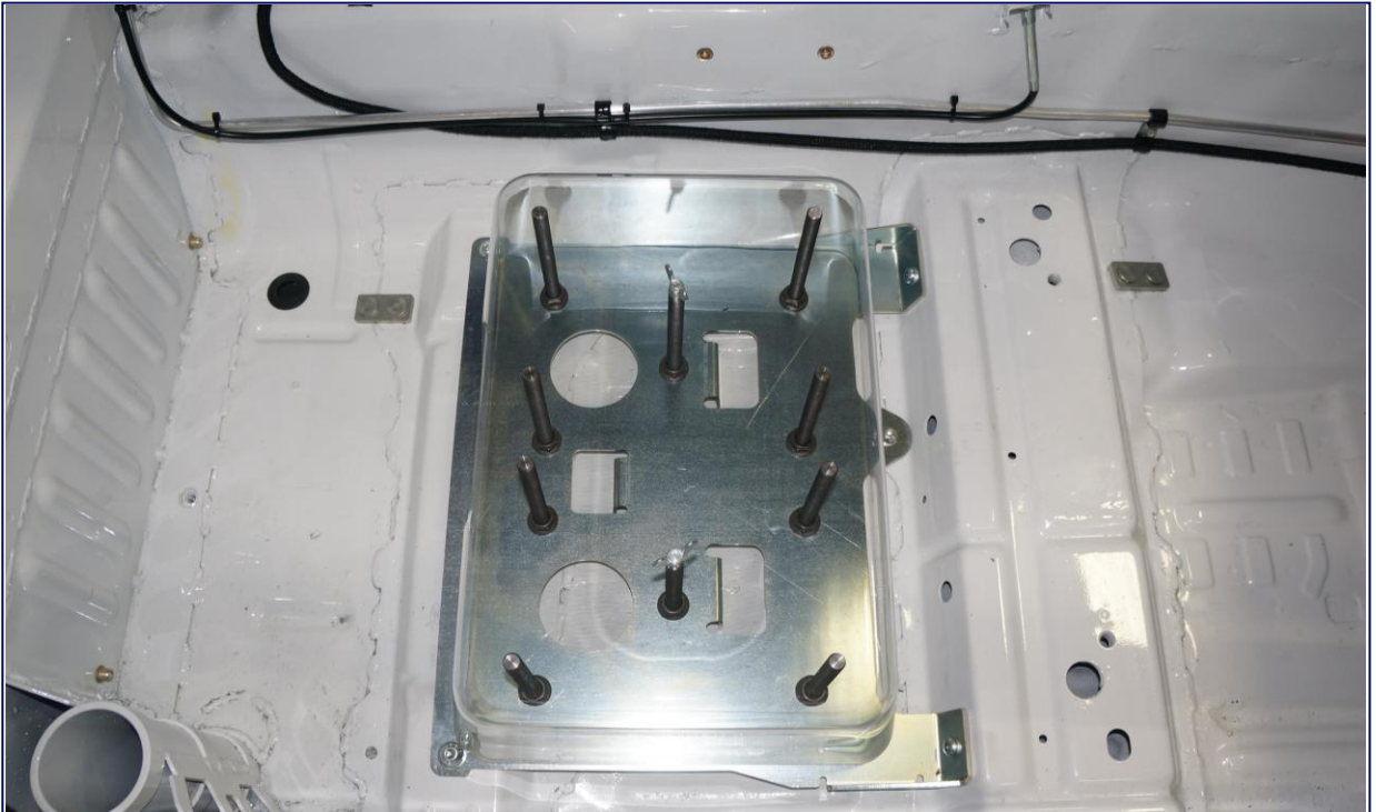
Ballast Assembly Location – Passenger Side Floor Ballast Assembly may be removed if not required
