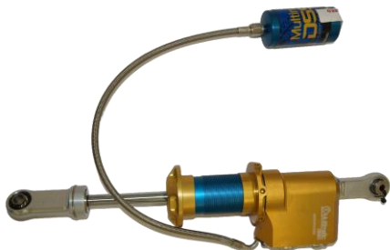
Rear Damper Assembly – LH/RH FP-18000R-DHR
