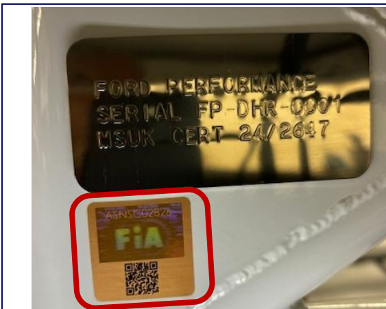
Safety Cage FIA Certification Standard (As Delivered)
