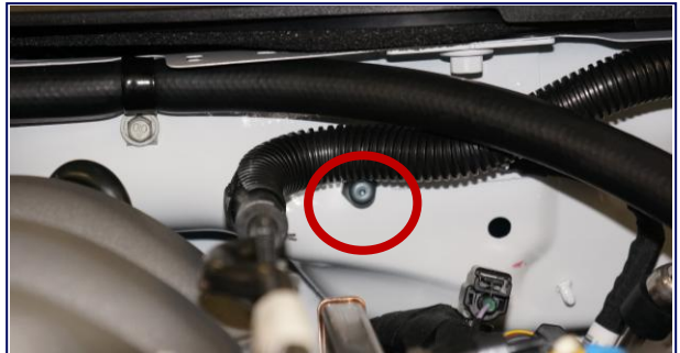
Engine Bay Nozzle 1 Driver Side
