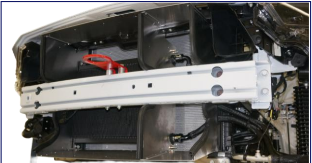
Radiator Closeout DHR-RADCLOSEOUT
