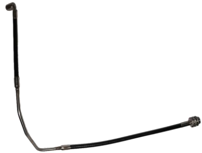
Front Brake Line – RH FORDM-B04
