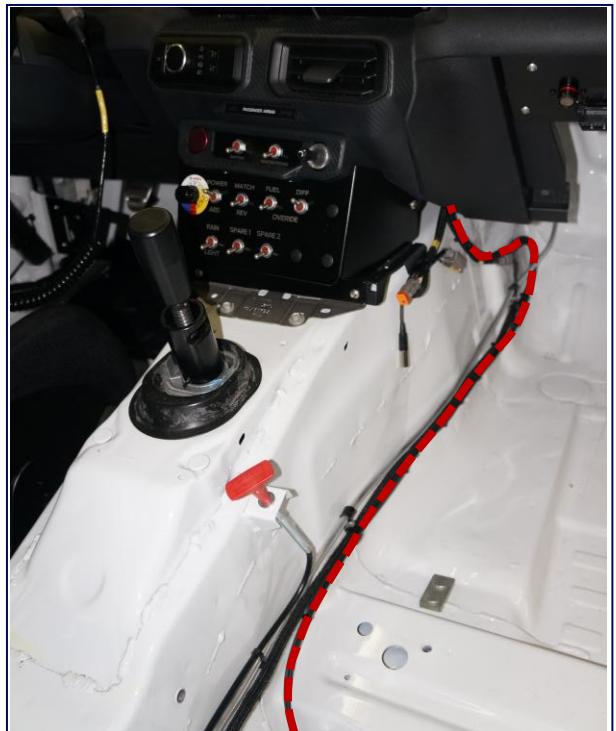
Safety System Routing Location Passenger Side
