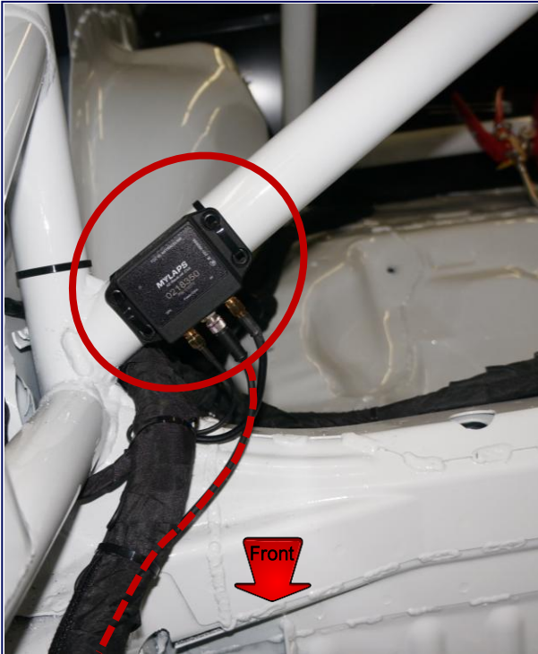
Safety System Location Passenger Side Roll Cage
