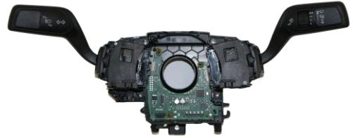
Multifunction Switch DHR-CLMNSWTCB-MOD
