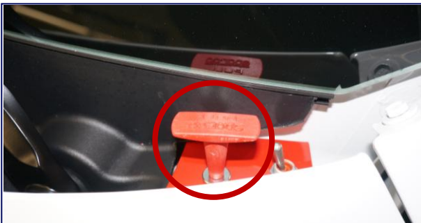
Exterior Cable Pull Exterior Driver Side
