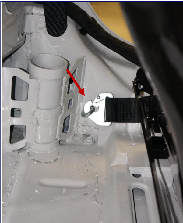
Harness Mounting Point Driver's Side Rear
