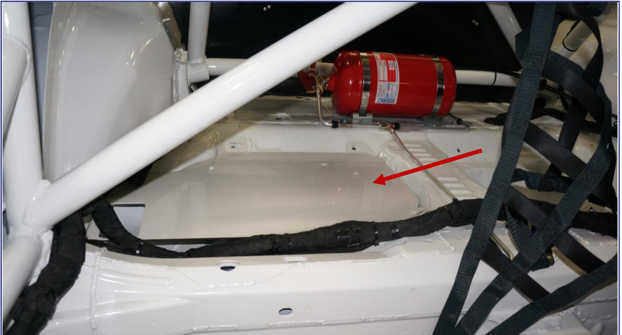
Driver Cooling System Mount* (Optional) 13052-09-1158 Passenger Side Rear Seat *Mount will be zinc-plated
