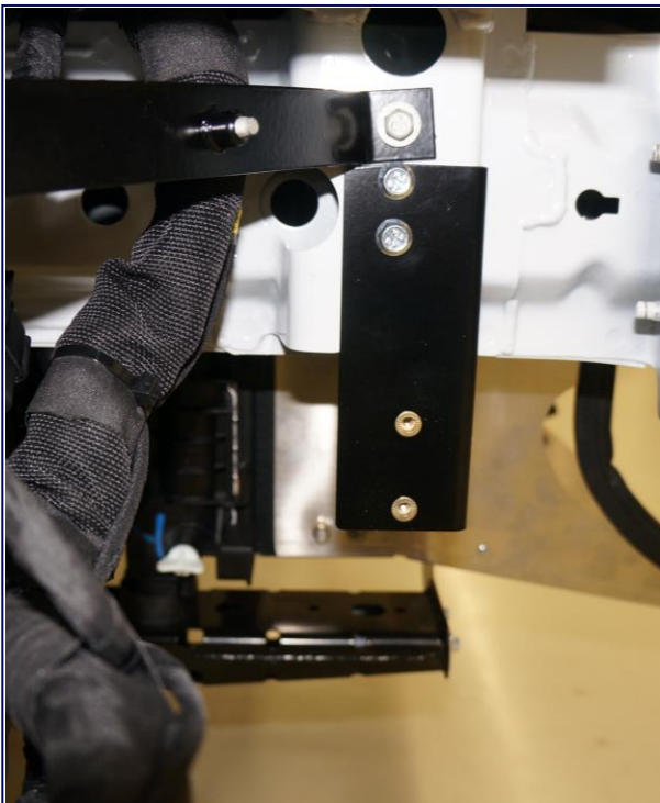
Transponder Bracket Location Front Passenger Side
