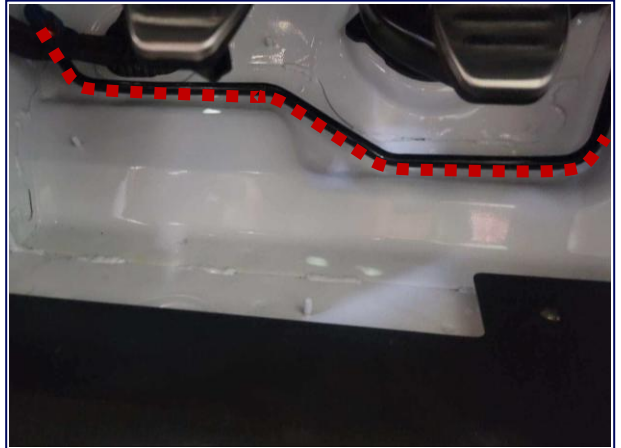
Front Air Jack Line Routing Driver Side
