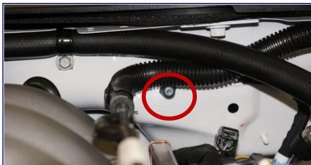
Engine Bay Nozzle 1 Driver Side
