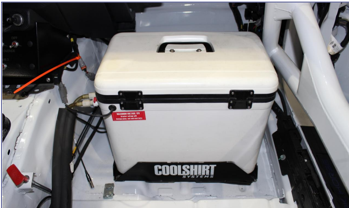
Driver Cooling System Location Passenger Side Footwell
