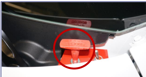
Exterior Cable Pull Exterior Driver Side
