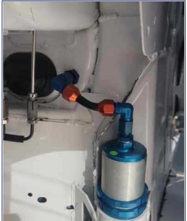
Front Air Jack / Bulkhead Connection Driver Side
