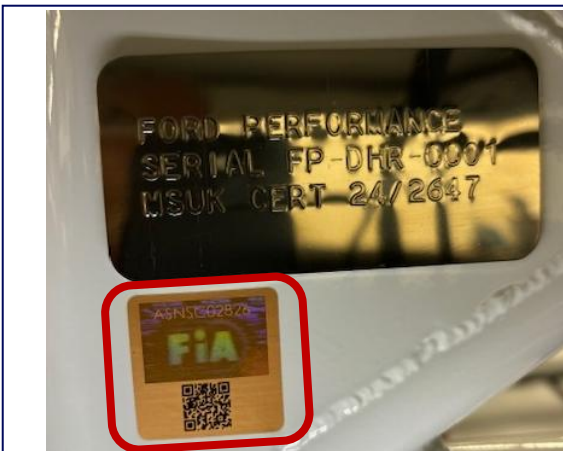
Safety Cage FIA Certification Standard (As Delivered)
