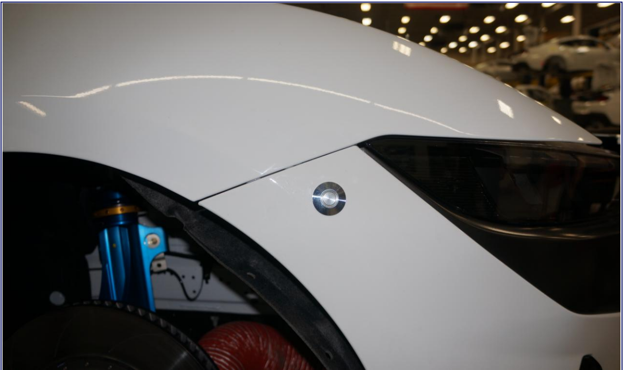
Front Fascia Mount Repair Only repair allowed for damaged front fascia corner mounts
