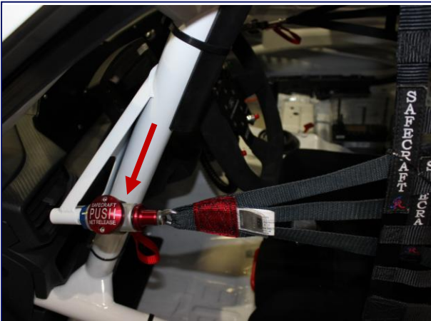
Driver Helmet Support Net Quick Release
