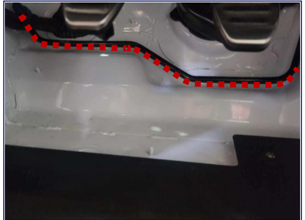
Front Air Jack Line Routing Driver Side
