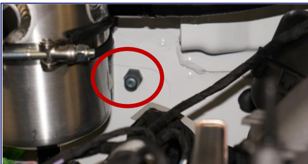
Engine Bay Nozzle 2 Passenger Side
