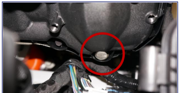
Engine Seal 3 Valve Cover RH Seal
