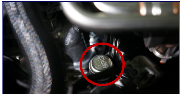
Engine Seal 4 Intake Manifold Seal
