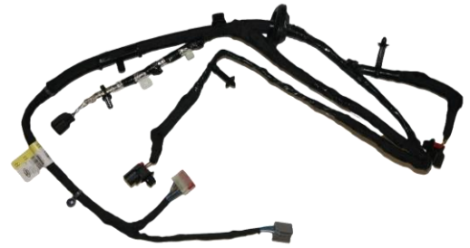
Diff Temp / Rear Chassis Harness PR3T-2B572-FFMOD
