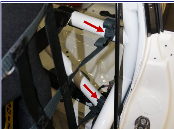
Driver Helmet Support Net Mounting Points
