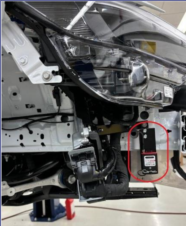
Transponder Location Front Passenger Side
