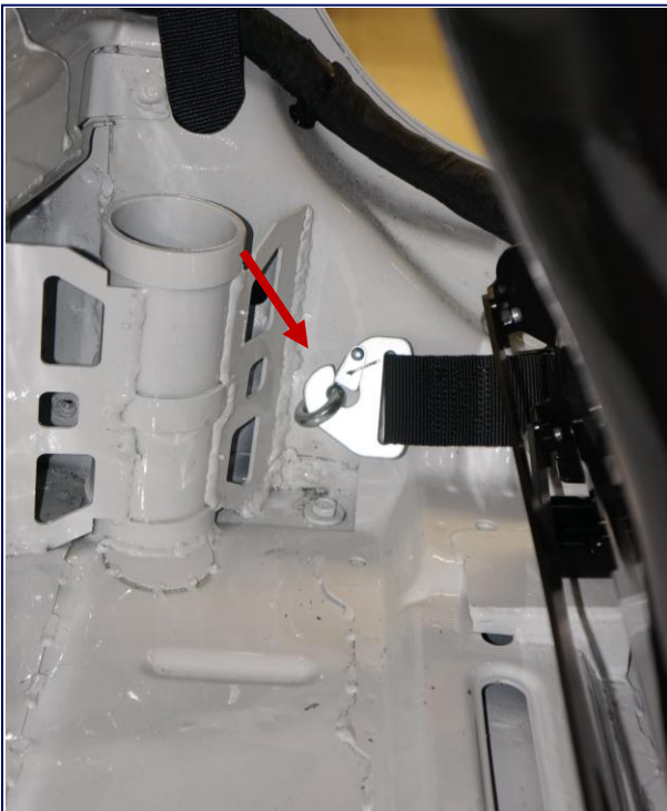
Harness Mounting Point Driver's Side Rear
