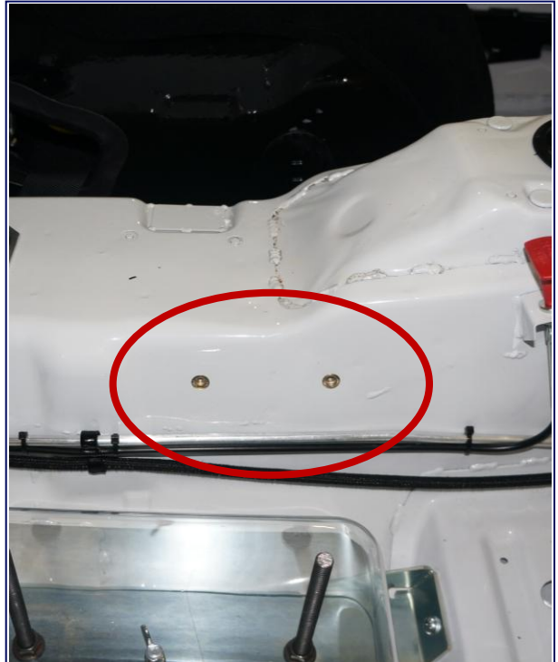
Radio Mounting Location (2) M6 Rivnuts Provided
