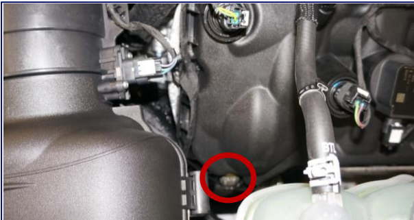
Engine Seal 2 Valve Cover LH Seal
