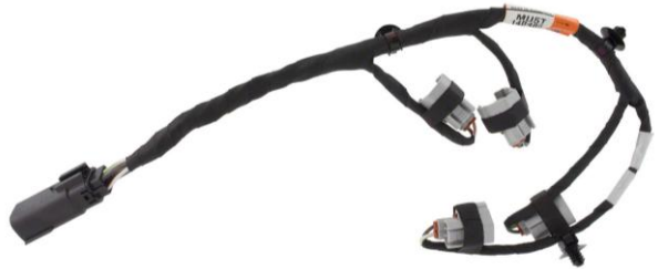
Fuel Injector (Direct) Harness BNK 2 – LH MU5Z-14A411-MA
