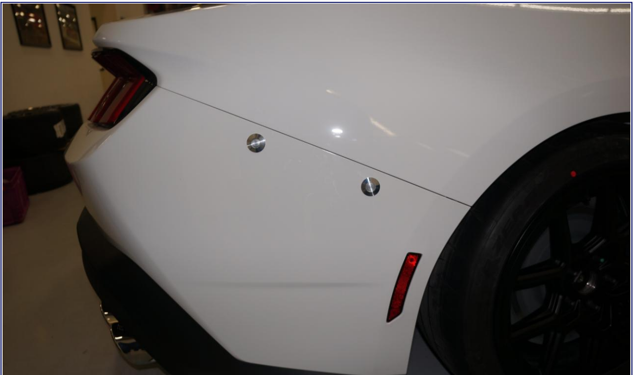
Rear Fascia Mount Repair Only repair allowed for damaged rear fascia corner mounts
