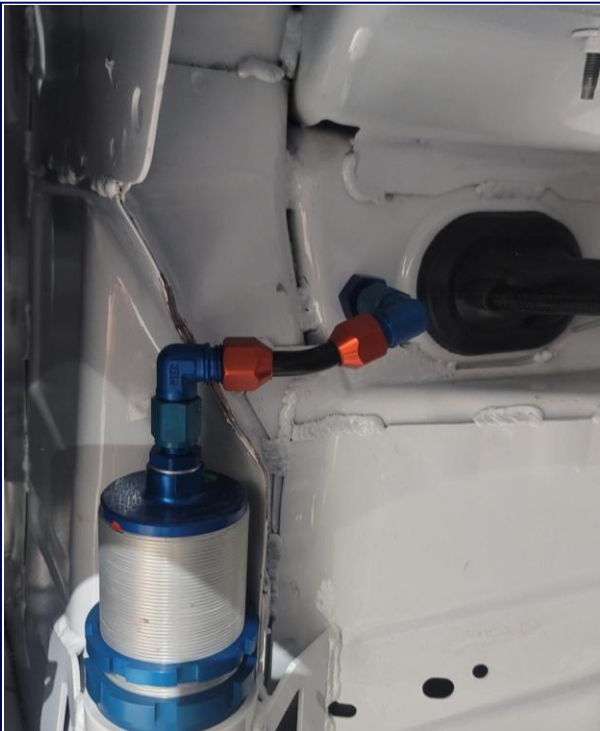
Front Air Jack / Bulkhead Connection Passenger Side
