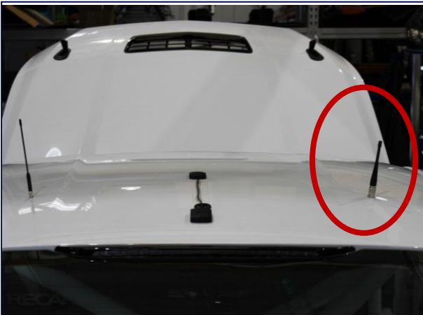
Antenna Location Passenger Side Roof
