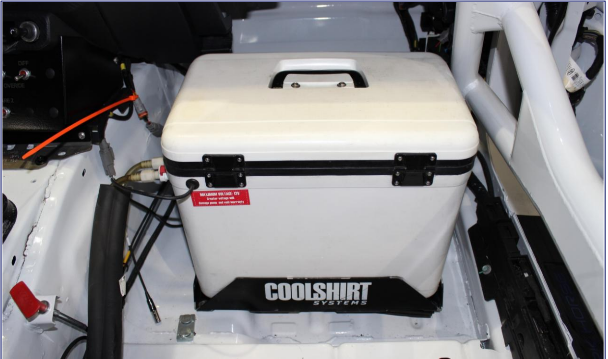
Driver Cooling System Location Passenger Side Footwell
