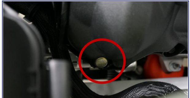
Engine Seal 2 Valve Cover LH Seal
