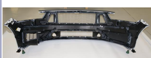
Front Fascia Assembly w/ Upper and Lower Grill Mesh FP-17000-DHR DHR-MESHGRL-UPR / DHR-MESHGRL-LWR
