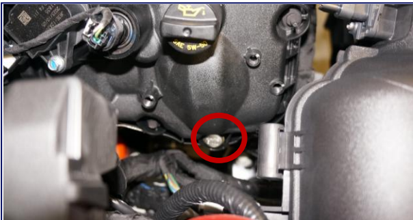
Engine Seal 3 Valve Cover RH Seal
