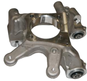
Knuckle / Bearing Assembly RH CM-5B758-S650
