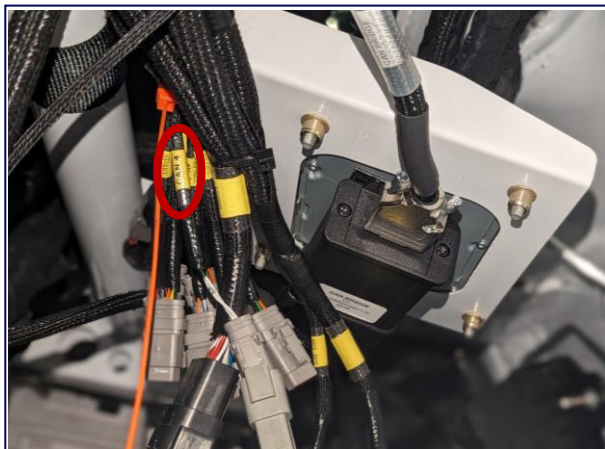
VBOX Wiring Labeled "CAN4" Underneath Dash
