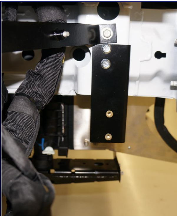
Transponder Bracket Location Front Passenger Side
