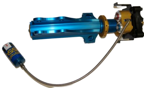
Front Damper Assembly – LH/RH FP-18000F-DHR
