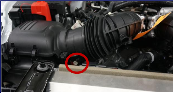
Engine Seal 1 Timing Cover Seal
