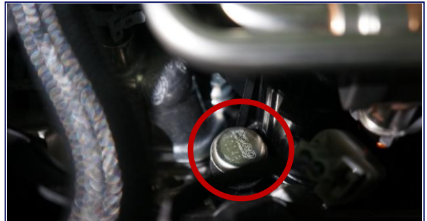
Engine Seal 4 Intake Manifold Seal
