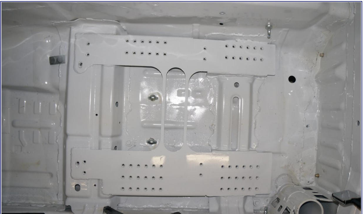
Standard Seat Mounting Plate for Cars 041-080 (Optional for Cars 001-040)
