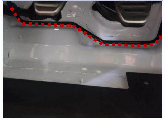
Front Air Jack Line Routing Driver Side
