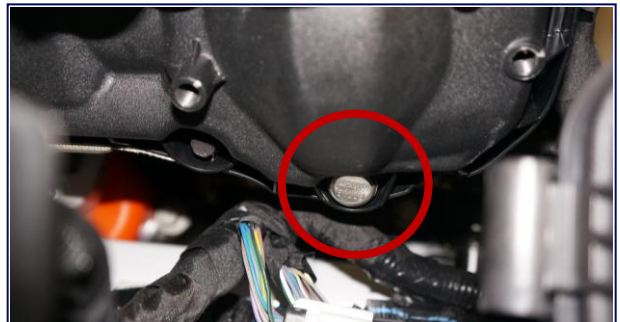
Engine Seal 3 Valve Cover RH Seal
