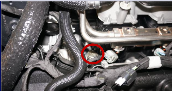
Engine Seal 4 Intake Manifold Seal
