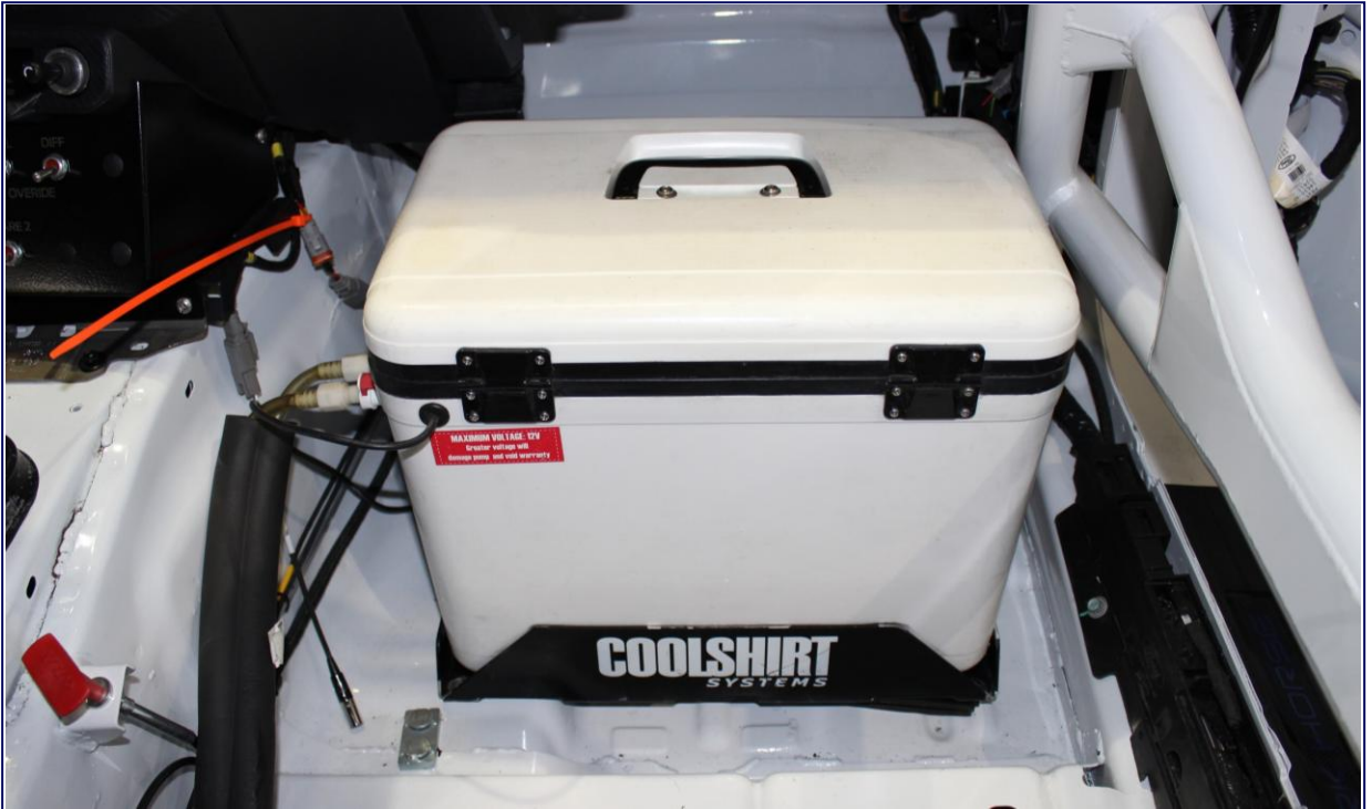
Driver Cooling System Location Passenger Side Footwell
