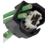
Variable Camshaft Timing (VCT) Solenoid AU2Z-14S411-DB
