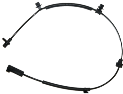
ABS Sensor - Front LH JR3C-2C204-B1B
