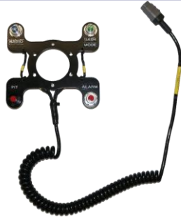
Steering Wheel Switch Plate / Harness FP-14A664-AA / DHR-STRNGWHLSWTCH
