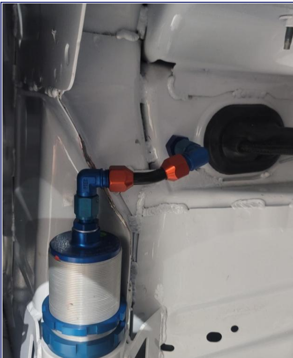
Front Air Jack / Bulkhead Connection Passenger Side
