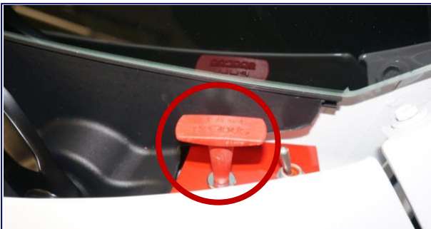
Exterior Cable Pull Exterior Driver Side
