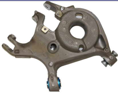
Rear Lower Control Arm LH DHR-RCNTRLBRNG-MODL
