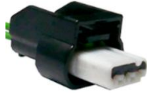
Engine Oil Pressure (EOP) HU2Z-14S411-BA
