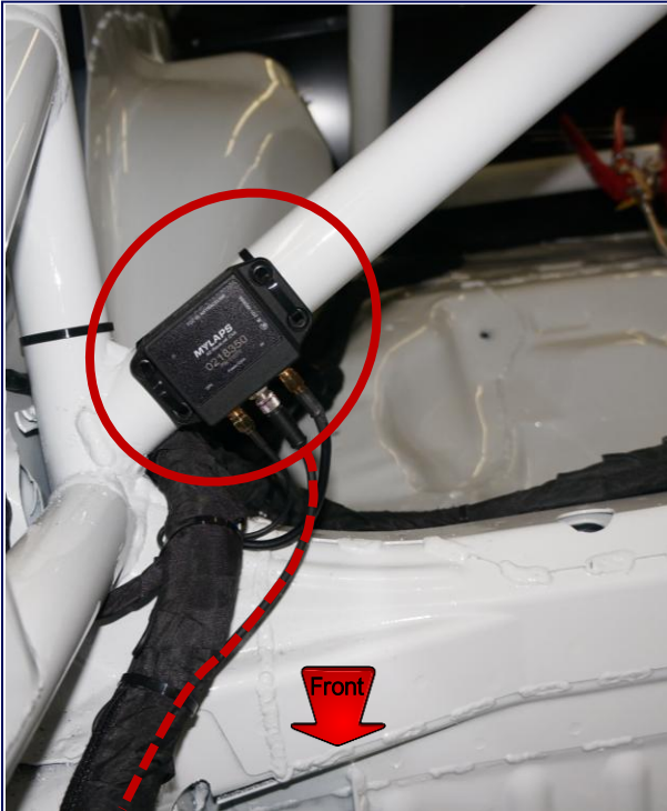
Safety System Location Passenger Side Roll Cage
