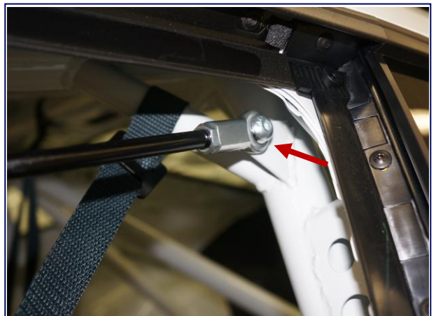
Driver Window Net Rod Mounting Point
