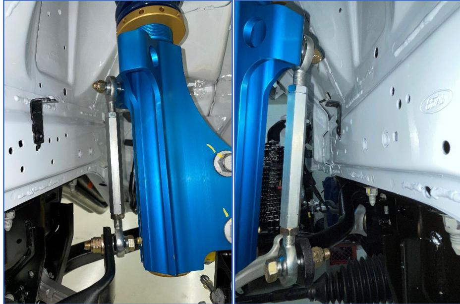
The large rod end and left-hand thread of the drop-link (denoted by the slots) attach to the ARB.
