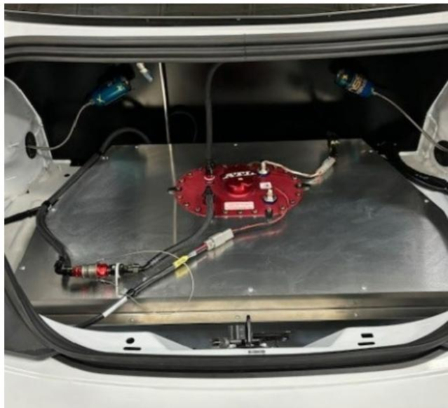
Fuel cell fill plate, M6-1, torque to 3.5 Nm (30 inlbf)
